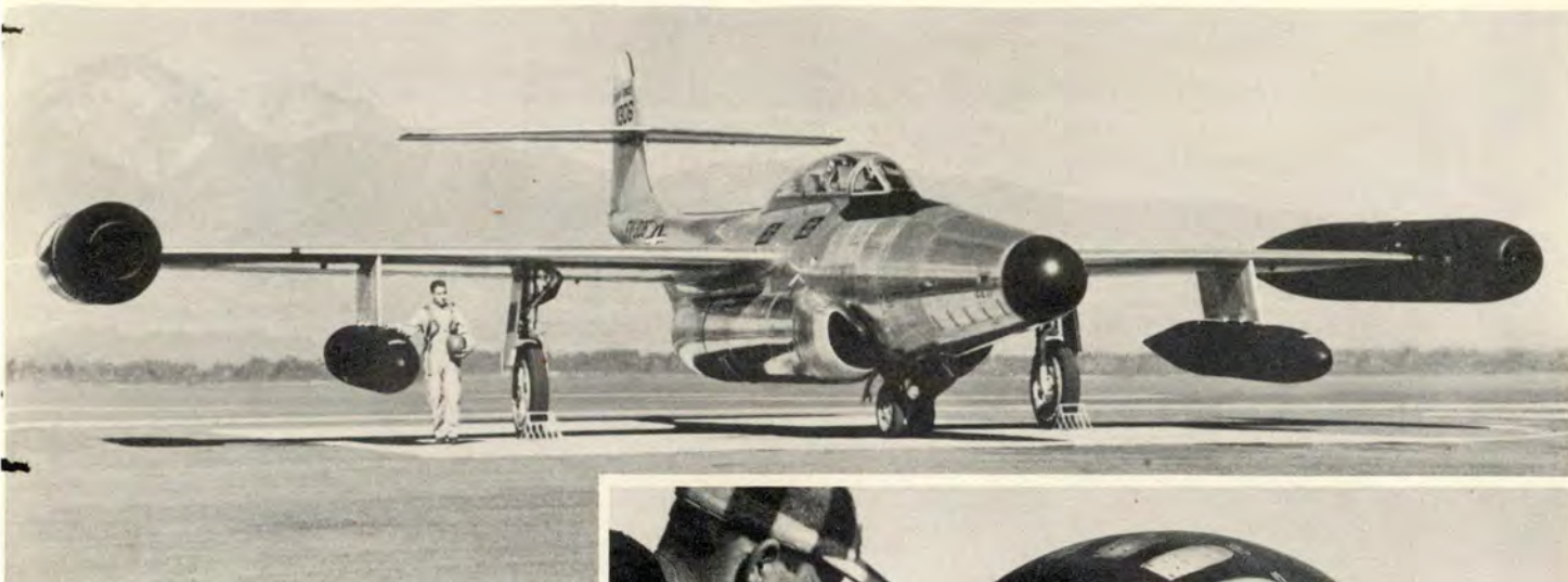
Above, the range of the F-89D is increased by jettisonable pylon tanks. Right, one of the twin pods is being loaded with 2.75 inch rockets. Each pod carries 52 rockets.
