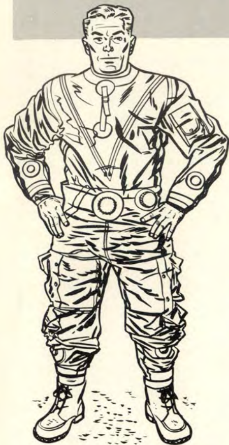
Air entrance assembly, with quick disconnect and sealing hose snapped over entrance port.
